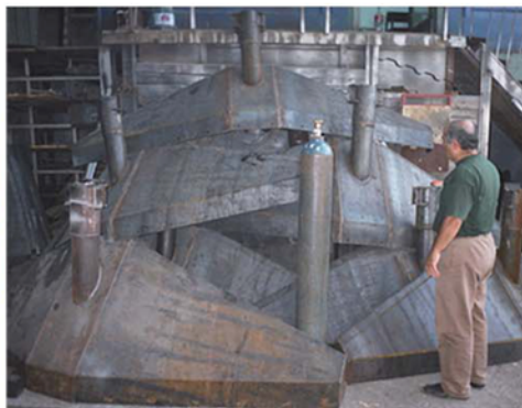
Suction type bottom scrapers ready for hot dip galvanizing.
